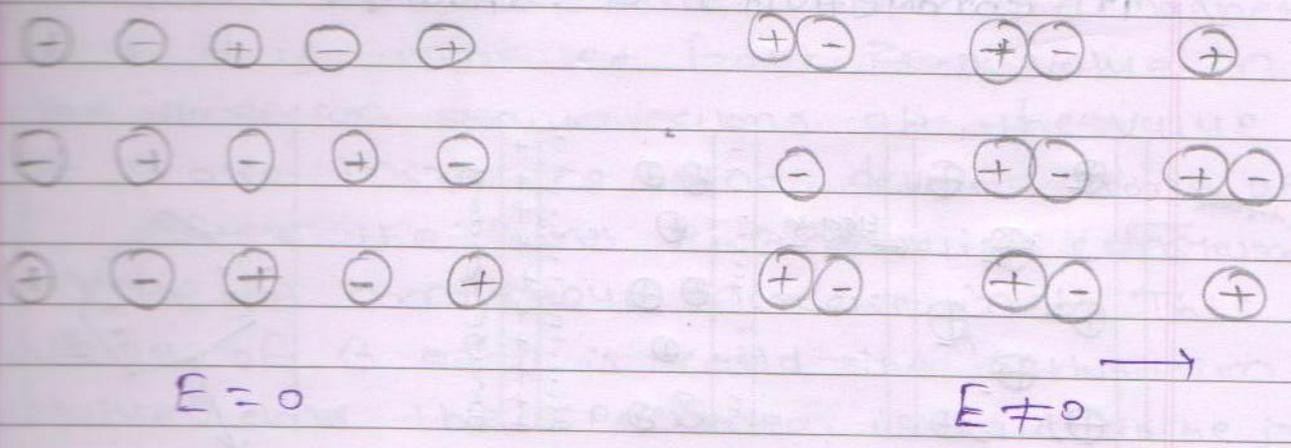
3) Orientation Polarisation: Orientation Polarisation occurs in dielectric materials which possess molecules with permanent dipole moment.
