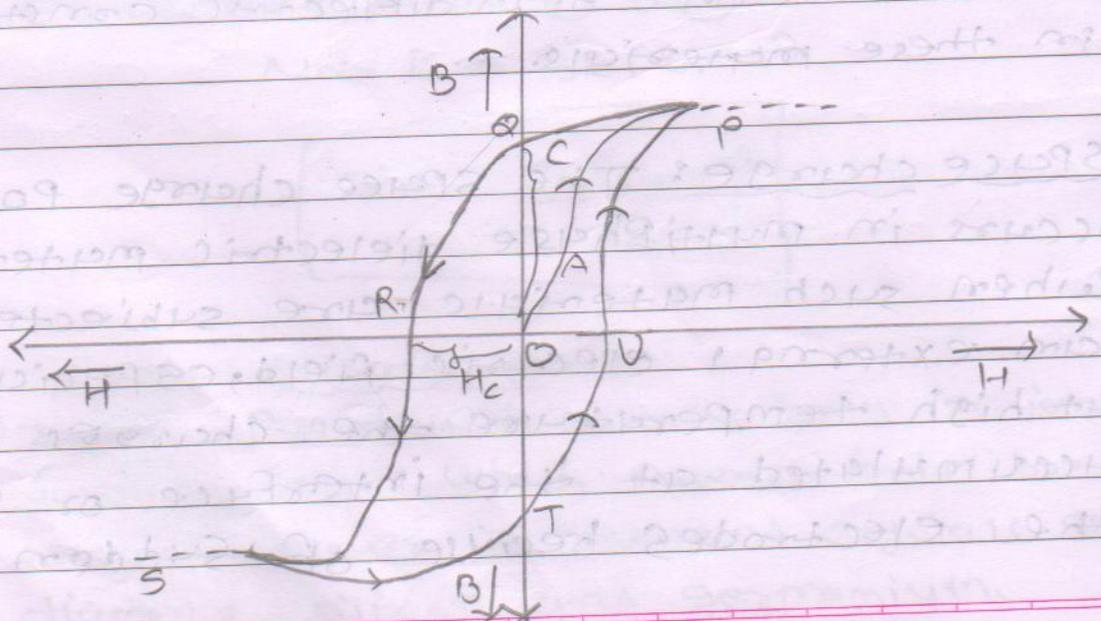
→ we can observe that when the magnetic field  $H$  is increased from zero value in the direction shown along  $OH$ , the value of  $B$  also increases and develops along  $OP$ .
