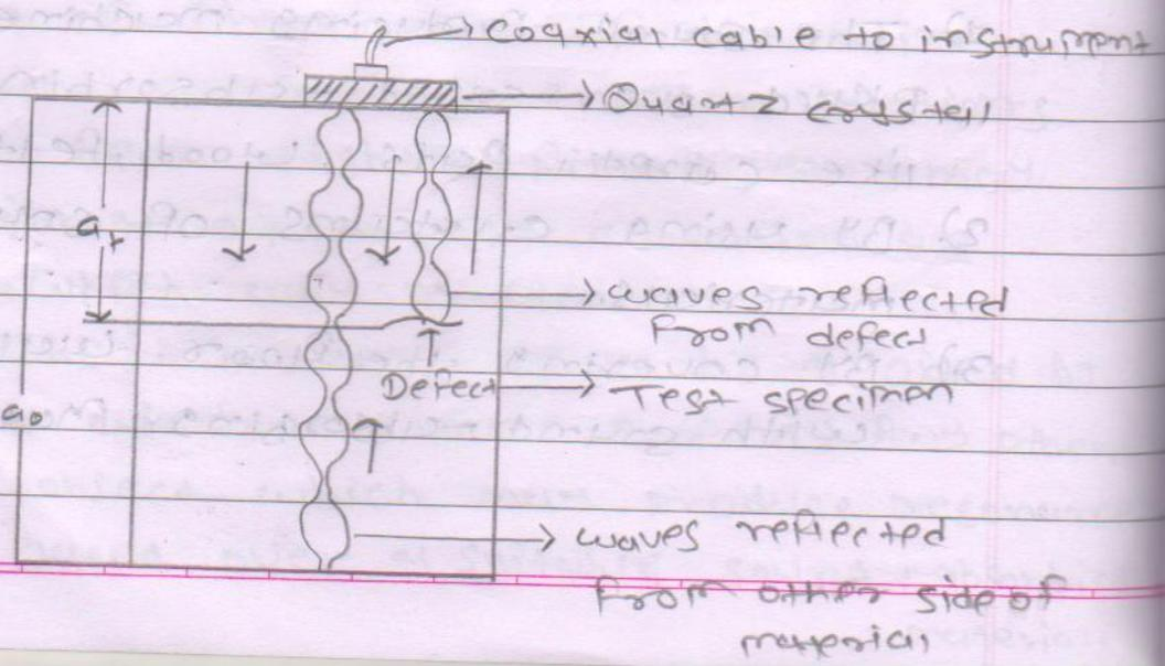
→ In the pulse echo system evenly timed pulses of ultrasonic sound waves are produced from a pulse generator which are transmitted into the material being tested.
