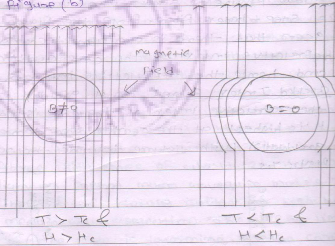
→ The above process occurs due to the development of surface currents, which in turn result in the development of magnetization in the superconducting material. Hence, the
