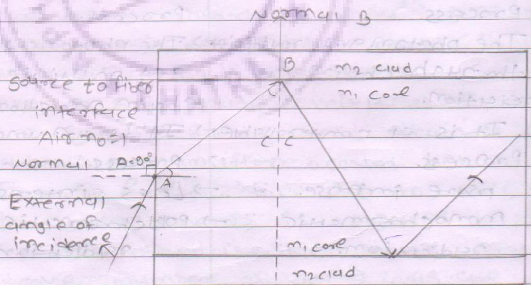
Light is launched into the end of the fibre from a launch region with a refractive index  $n_0$ . If the launch region is air then  $n_0=1$ . When light rays enter the fibre, they
